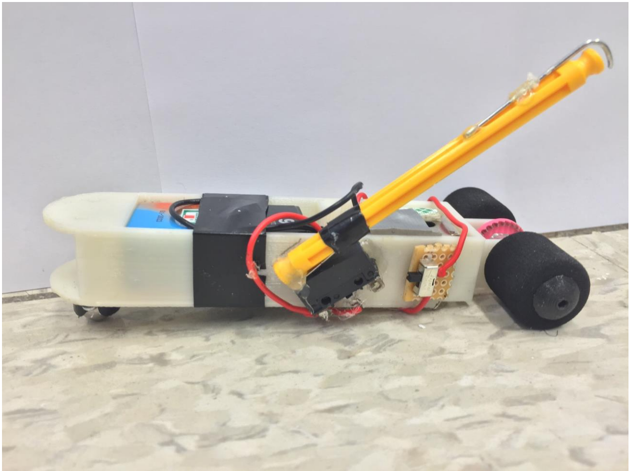
Photo 4: Completed pipe racer, with rounded hubcaps and limit switch activation arm
